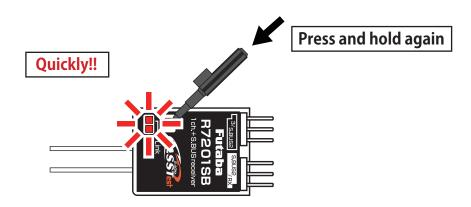
7. Release the switch when the solid orange.
