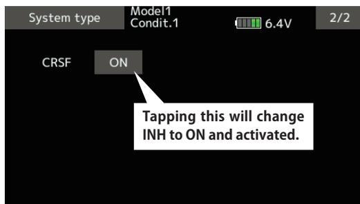
② Tap the "CRSF" button to [ON]. A signal conforming to the CRSF standard is output from the S.BUS setting connector (S.I/F) of the transmitter.
