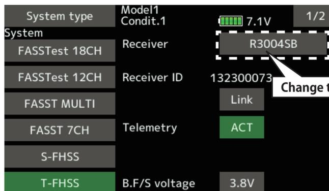
R3004SB receiver does not support model ID function.
